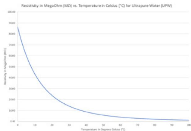
Graph above shows relationship between the resistivity of pure water at various temperatures. Computed resistivity MegaOhm (MΩ) units are the inverse of measured conductivity and so are the mirror image of the conductivity at various temperatures for ultrapure water (UPW). The graph above shows absolute raw resistivity at various temperatures. Resistivity values sent include ATC referencing reading to 25 °C state.
