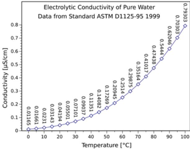
The conductivity of pure water varies significantly with temperature in a well defined but non-linear fashion as detailed in the graph to left. This behavior is preprogrammed into the DSS-CON-L Modbus RTU conductivity sensors for the automatic temperature compensation feature to make it suitable for ultrapure water (UPW) type applications.
