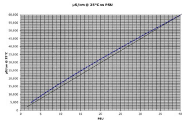
Salinity computed from the measured conductivity. Curves that define the relationship between measured conductivity and the computed salinity in PSU are preprogrammed into the sensor with a full range of 0.000 to 50.000 PSU.
